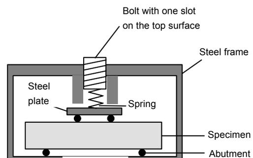
Fig. 3 Sketch of the small-sized preloading setup
