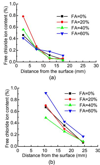
**Fig. 5** Effect of fly ash content (FA) on 1D (a) and 2D (b) chloride ion diffusion of concrete under flexural stress with the stress ratio of 0.35
