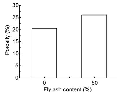
**Fig. 6** Effect of fly ash content on porosities of concrete
