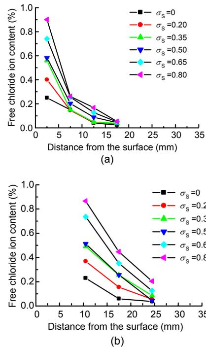
**Fig. 11** Effect of stress ratios ( $\sigma_s$ ) on 1D (a) and 2D (b) chloride ion diffusion of concrete
