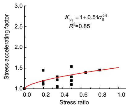
**Fig. 13** Relationship between the stress accelerating factor and the flexural stress ratios
