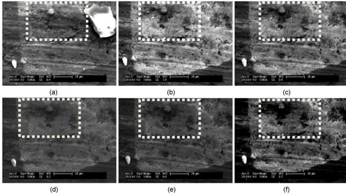
**Fig. 12** In-situ SEM observations of the microcrack prorgation on the tensile faces of specimen under different stress ratios: 0 (a), 0.2 (b), 0.35 (c), 0.50 (d), 0.65 (e), and 0.80 (f)
