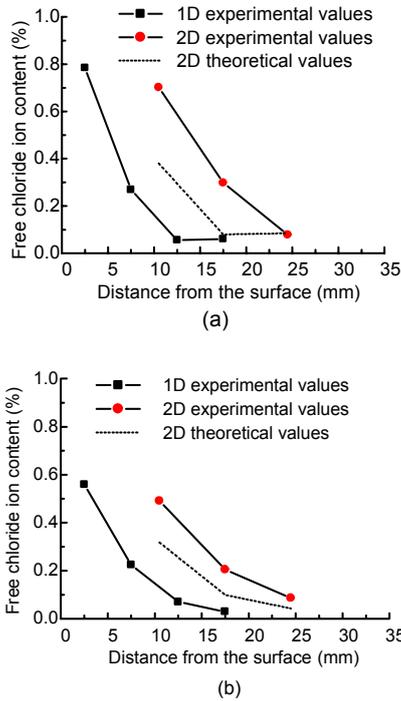
**Fig. 9** Effect of dimensions on chloride ion diffusion of fly ash concrete under flexural stress
