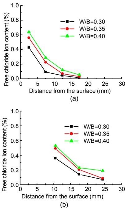
**Fig. 7 Effect of water to binder ratio on 1D (a) and 2D (b) chloride ion diffusion of concrete under flexural stress with the stress ratio of 0.35**
