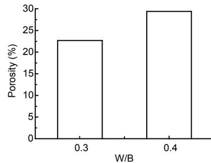
**Fig. 8 Effect of W/B on porosities of concrete**
