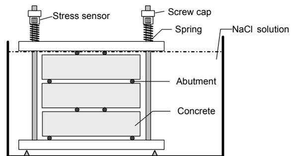
**Fig. 1** Sketch of the preloading concrete subjected to 1D and 2D chloride ion attacks
