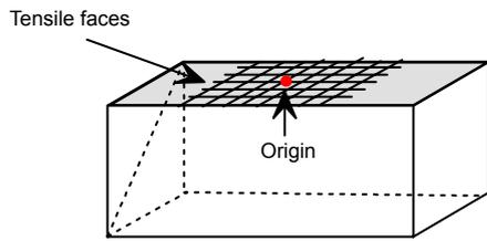
**Fig. 4** Microcracks observation locations on the tensile faces of specimen under flexural stress
