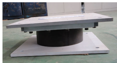
Fig. 6 Model of the multi-functional bridge seismic isolation bearing (MFBSIB)
