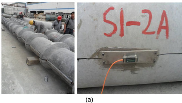
Fig. 6 Sketch of strain gauges attached on pile (a) and schematic of the test (b)
