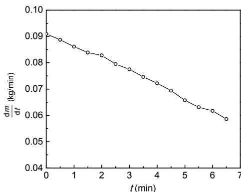
Fig. 9 Ice production rate in 10% EG solution
