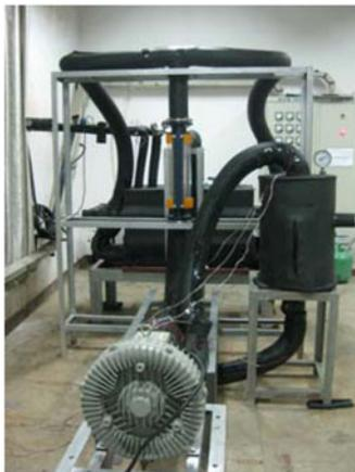
Fig. 4 Prototype of ice slurry making system
