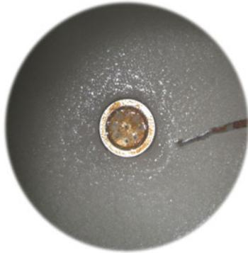
Fig. 8 Ice slurry formation around the nozzles
