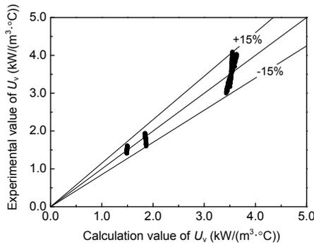
Fig. 3 Correlation results of volumetric heat transfer coefficient
