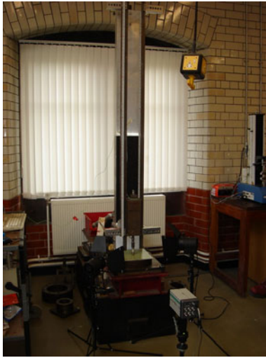
Fig. 1 The drop-weight rig used for characterising the dynamic properties of samples
