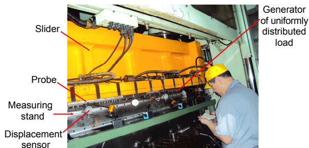
Fig. 9 Measurement of prototype's linear deflection
