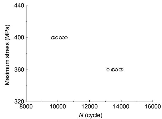
Fig. 4 The S-N data of corrosion fatigue
