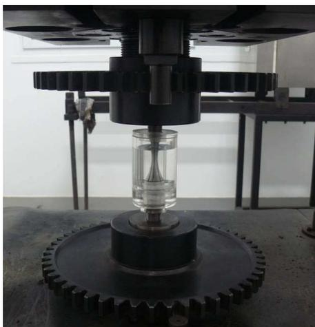
Fig. 3 Loading equipment for corrosion fatigue
