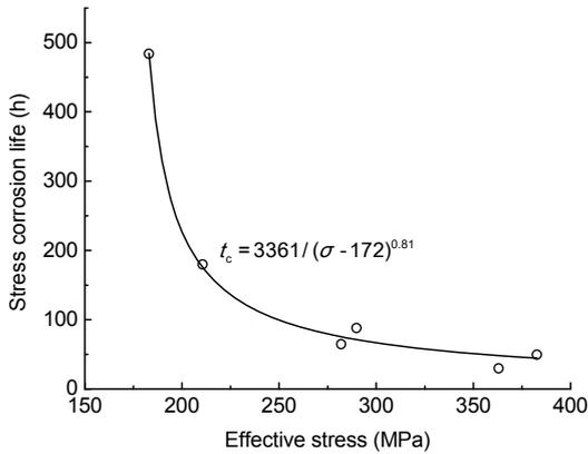
Fig. 2 Stress corrosion life curve of LY12CZ aluminum
