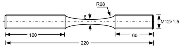
**Fig. 1 Schematic diagram of funnel-shaped specimen (unit: mm)**
