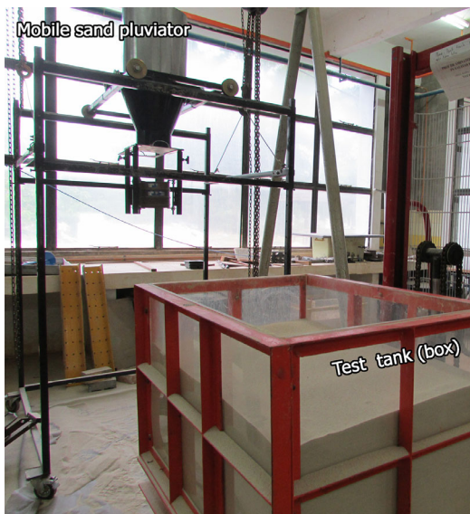
Fig. 6 Mobile sand pluviator and test tank
