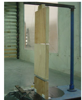
Fig. 7 Arrangement of the sectional model in the wind tunnel
