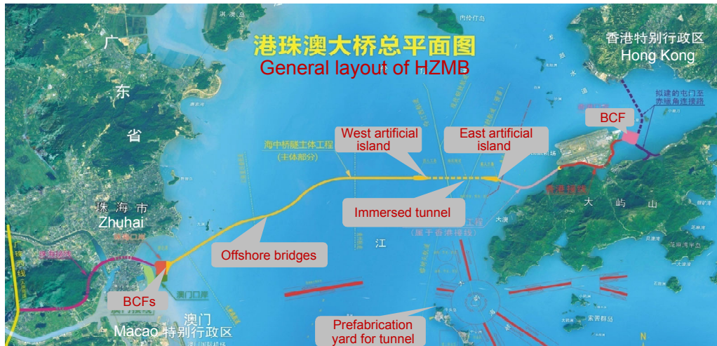
Fig. 1 General layout of the HZMB BCF: boundary crossing facility
