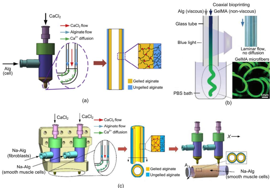
**Fig. 3 Schematic illustration fabrication by coaxial bioprinting**
