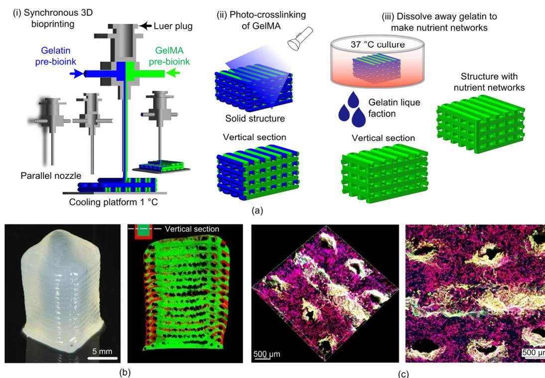
**Fig. 5** 3D bioprinting strategy for engineering large-scale tissue constructs with nutrient networks (a); 3D bioprinting multi-compartmental construct and its vertical sections (b); confocal laser scanning microscopy (CLSM) images of the vascularized osteogenic tissue constructs (c)
