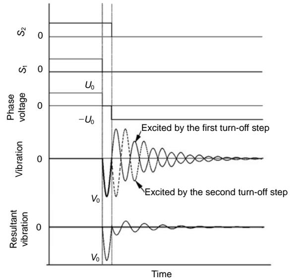
Fig. 2 The principle of active vibration cancellation
