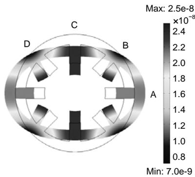
**Fig. 6 Deformation with phase C winding excitation (excitation force=5000 N/m<sup>2</sup>)**
