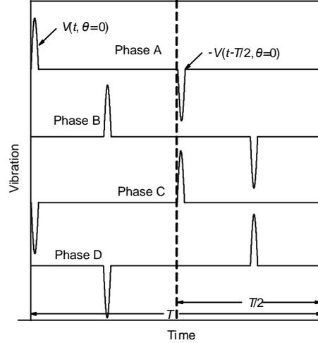
Fig. 5 Schematic diagram of stator vibration by applying active vibration cancellation (AVC)
