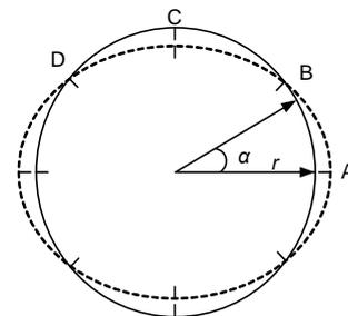
Fig. 3 Elliptical deformation in an 8/6 switched reluctance machine
