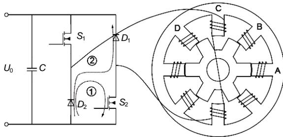
Fig. 1 A four-phase 8/6 switched reluctance machine and one phase leg of an asymmetric bridge inverter
