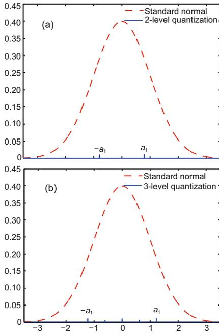
**Fig. 2** Schematic of 2-level (a) and 3-level (b) quantization
