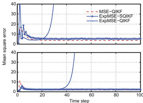
Fig. 9 Mean square errors (MSEs) of 2-level (a) and 3-level (b) QIKF and SQIKF in Example 3. For 2-level SQIKF,  $\tau_1 = 1.3634$ ,  $\tau_2 = 1.8$ ; for 3-level SQIKF,  $\tau_1 = 1.1902$ ,  $\tau_2 = 1.3$
