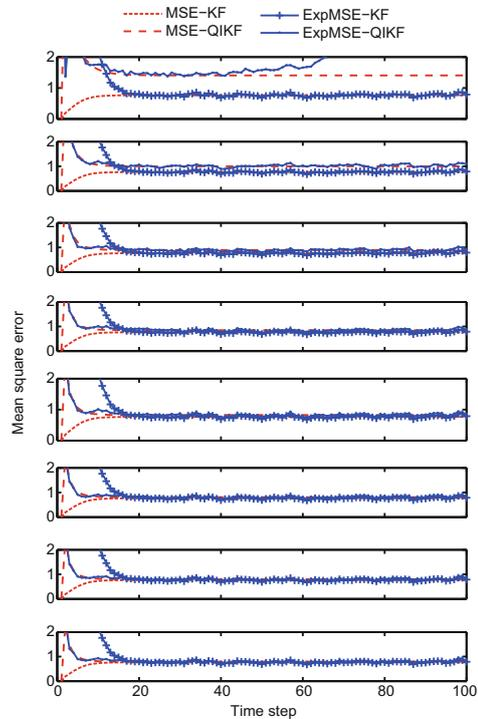
**Fig. 3** Mean square errors (MSEs) of 2-, 3-, ..., and 9-level (in increasing order of the number of levels from top to bottom) KF and QIKF in Example 1 ( $a = 1.15$ )
