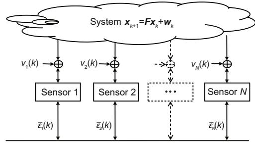
Fig. 1 State estimation with quantized innovations
