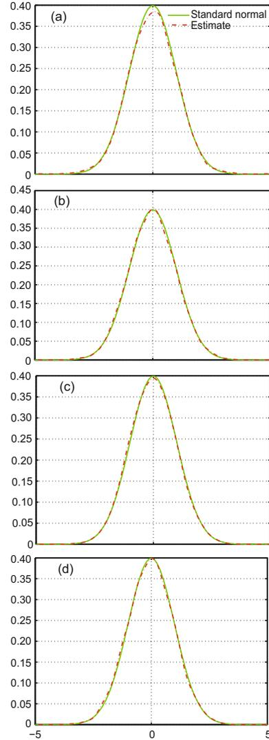
**Fig. 5** Probability density estimation of normalized innovations for 2-level (a), 3-level (b), 4-level (c), and 5-level (d) quantization in Example 1 (time step=40)
