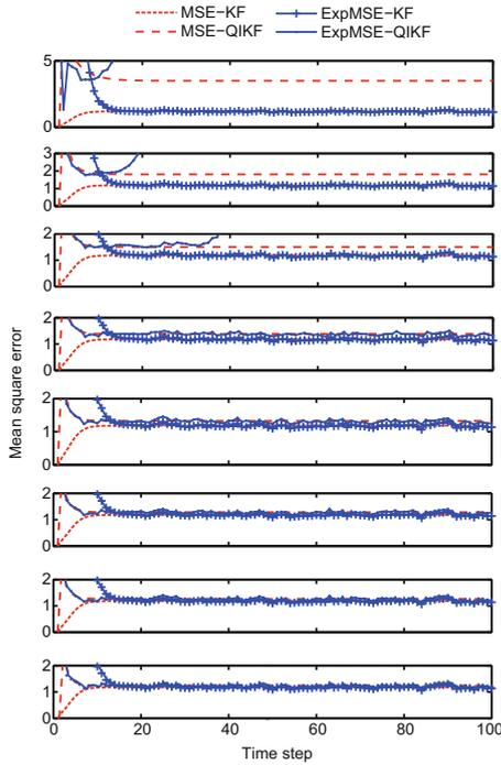
**Fig. 4** Mean square errors (MSEs) of 2-, 3-, ..., and 9-level (in increasing order of the number of levels from top to bottom) KF and QIKF in Example 1 ( $a = 1.35$ )
