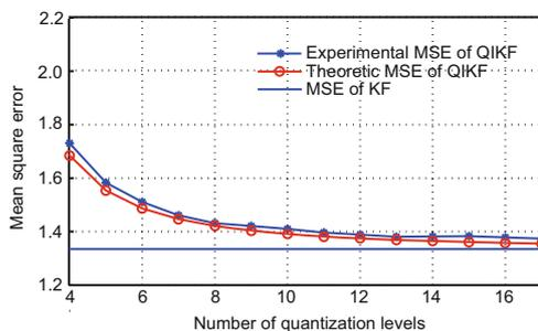
Fig. 8 Limits of the mean square error (MSE) in Example 2
