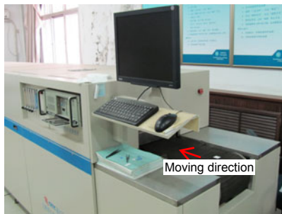
Fig. 11 Furnace for air outlet sealing
