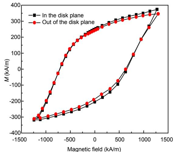
**Fig. 4** Demagnetization curves of a resin-bonded NdFeB micromagnet
