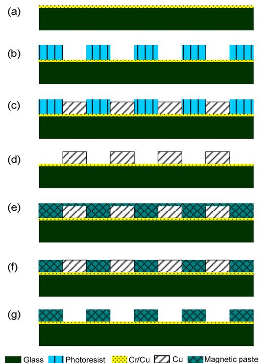
**Fig. 2** Fabrication process for resin-bonded NdFeB micro magnets
