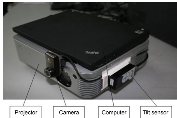
Fig. 10 Prototype of the intelligent projection system
