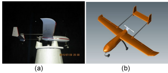
Fig. 12 The measured Pioneer UAV data experiment: (a) target model; (b) imaging scene in the microwave chamber
