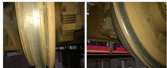
Fig. 4 Wheel wear photographs from a light rail train
