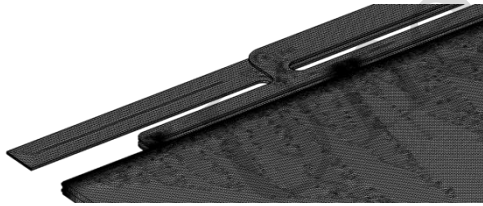
Fig. 4 Mesh refinement in the corners
