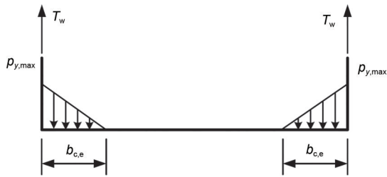
Fig. 7 Simplified distribution of the lateral stress and equivalent width of the area experiencing compression
