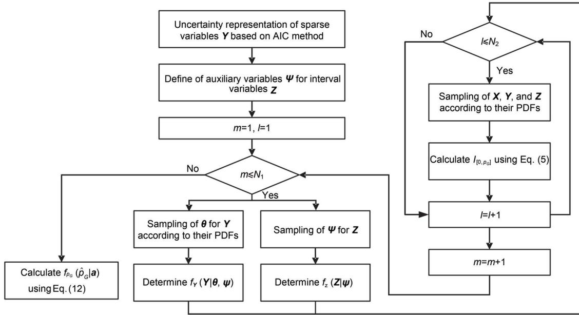
Fig. 2 Calculation flow chart for failure probability. AIC is the Akaike information criterion
