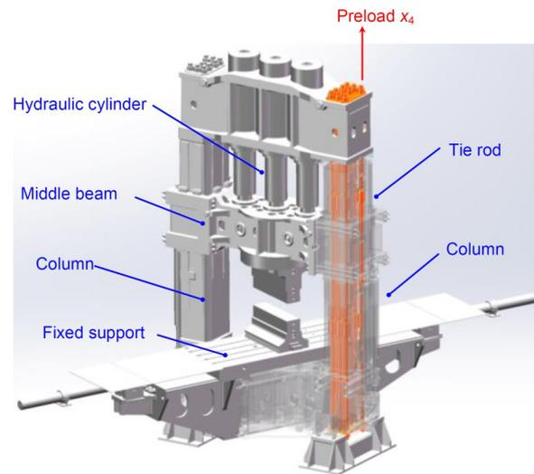
**Fig. 10 Forging hydraulic press**
