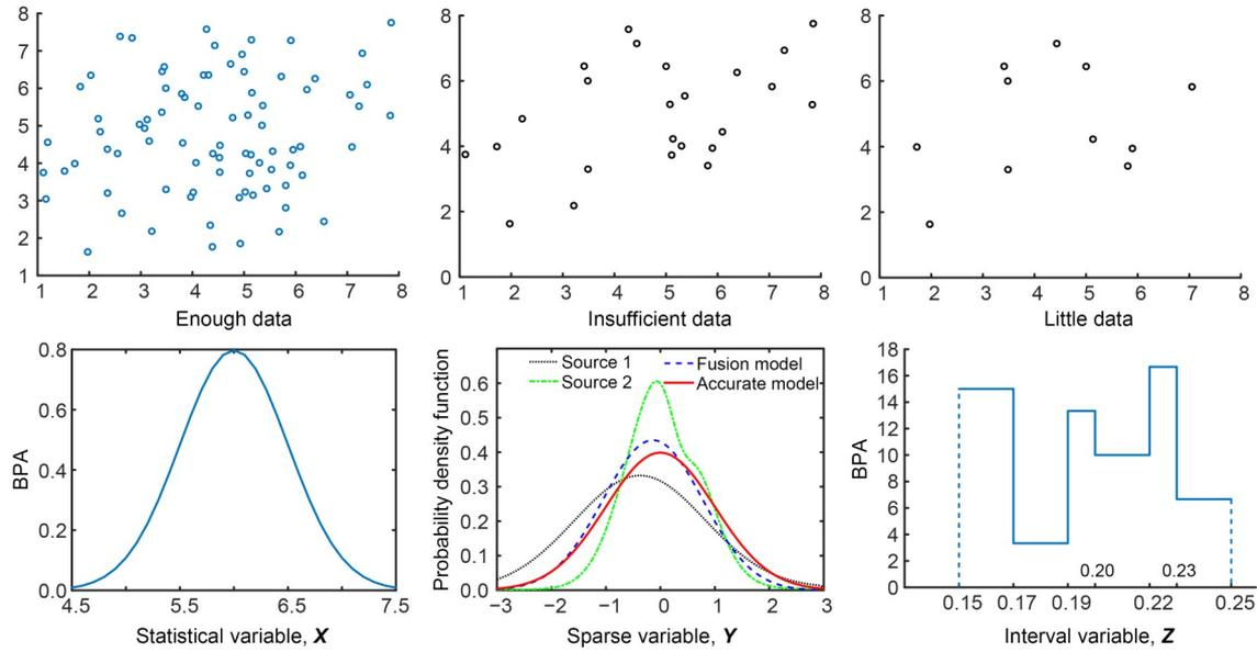
Fig. 1 Multiple uncertainty types due to insufficient input data. BPA represents basic probability assignment
