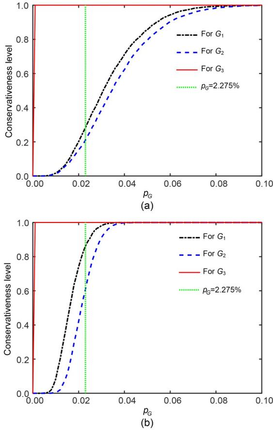
**Fig. 3** Conservativeness level of failure probability considering sparse variables: (a) 10 input data; (b) 100 input data
