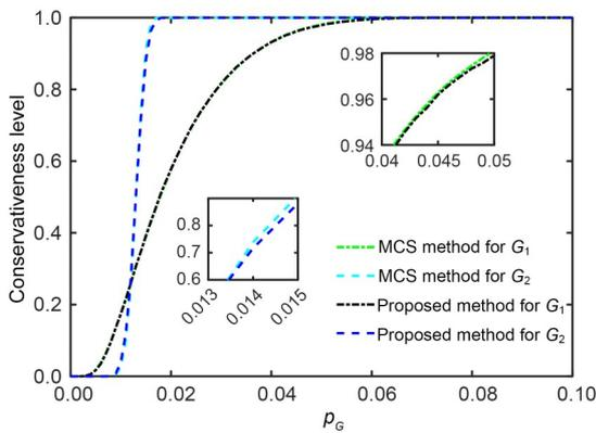
Fig. 6 Conservativeness level of failure probability of proposed method and MCS method
