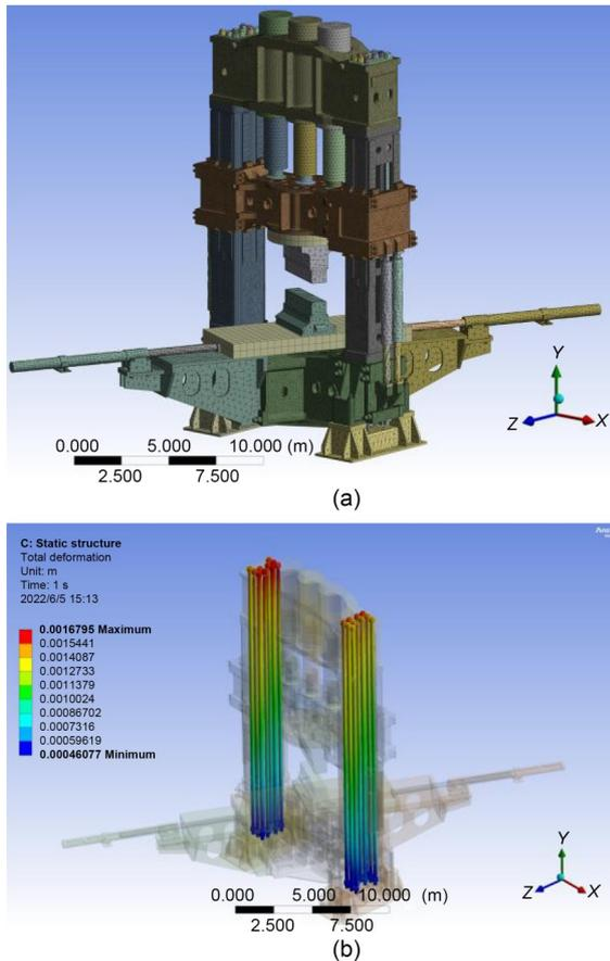
**Fig. 11 FEA of the forging hydraulic press: (a) mesh; (b) deformation of the tie rods**
