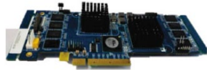
Fig. 4 High-throughput many-core processor DPU chip
