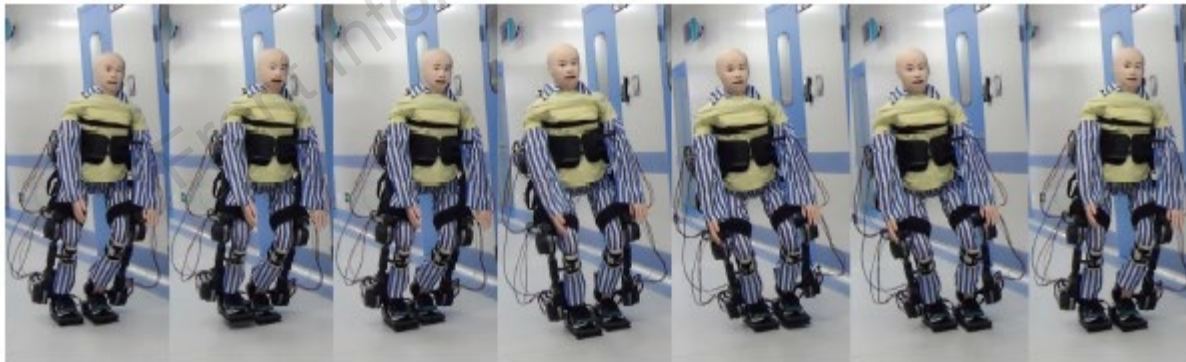
Fig. 16 Snapshots of self-balanced walking experiment with a dummy on a flat terrain
