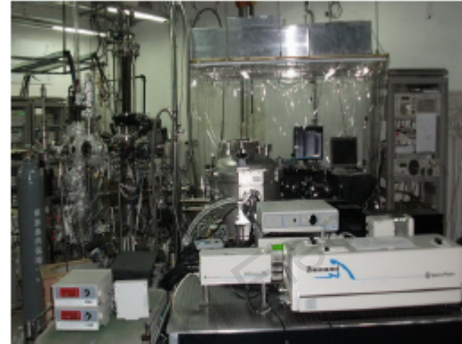
Fig. 29 Entity photo of super high energy and momentum resolution ARPES prototype based on DUV-DPL with 177.3 nm fixed wavelength and DUV-DPL with 175–210 nm widely tunable wavelength
