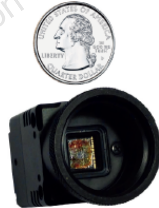
Fig. 14 A quantum dot micro-spectrometer in the form of a digital camera with electronics and circuits
