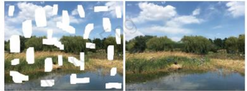
Fig. 8 Visual results of image inpainting. The masked area is shown in white
