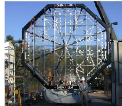
Foldable diffraction main mirror with aperture of 5 m
