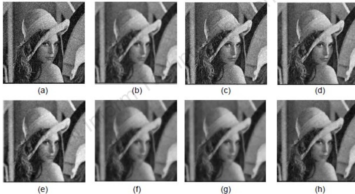
Fig. 3 Noise image (a) and the denoising effect obtained by the mean denoising method (b), Gaussian method (c), Wiener method (d), G-L method (e), PDE method (f), NLM method (g), and the proposed method (h)
