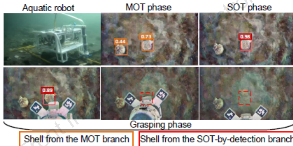
Fig. 11 Our robotic visual perception framework in the object grasping task. The proposed framework can provide robust visual information with visual restoration and flexible detection and tracking for robotic search and grasping
