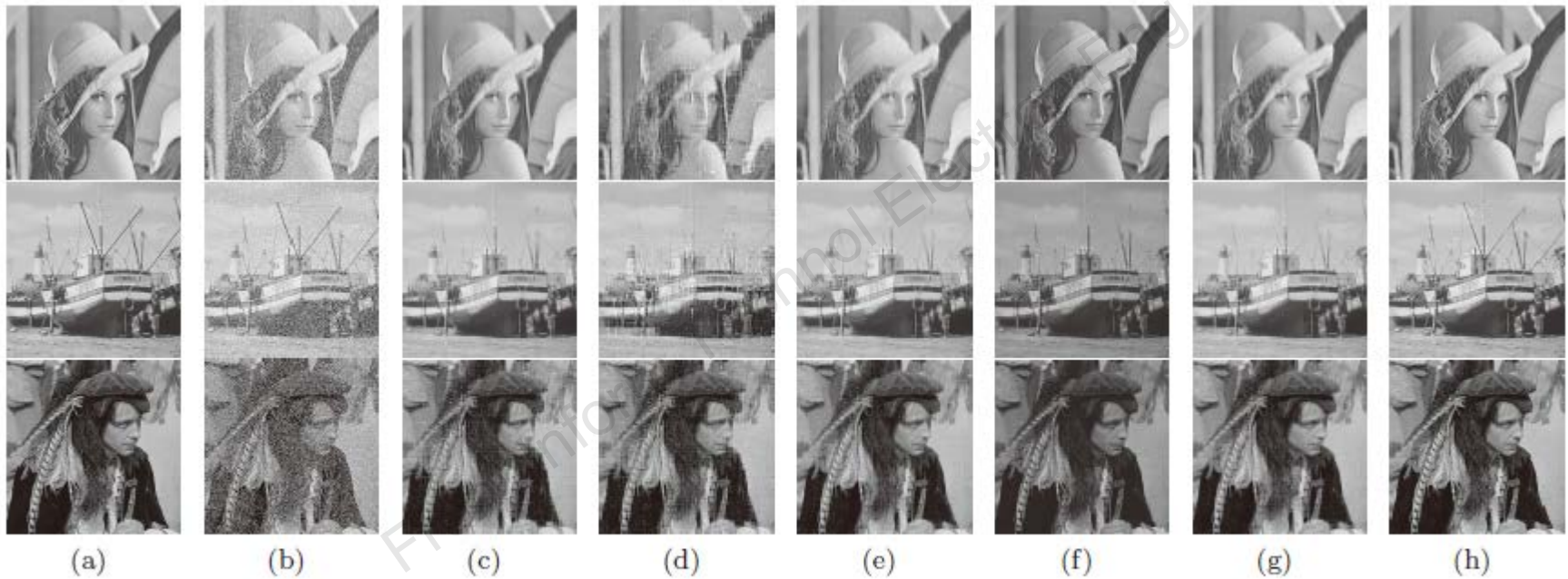
Fig. 5 Reconstruction results of the six algorithms for images with 20% salt and pepper noise: (a) original; (b) noisy; (c) PCP; (d) reweighted L_1 ; (e) NSVT; (f) ROUTE; (g) SRLRMR; (h) LRTGV
