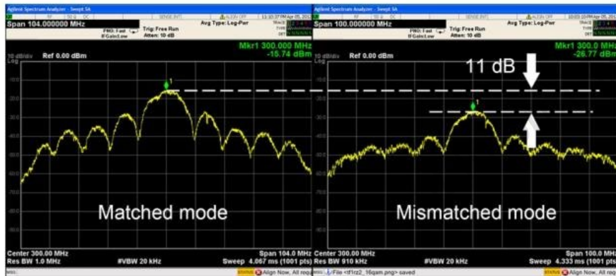
Fig. 7 TX OAM mode-checking: an 11-dB difference in intermediate frequency (IF) power. The TX mode is +1 while the RX UCA is -1 (matched) and +1 (mismatched)
