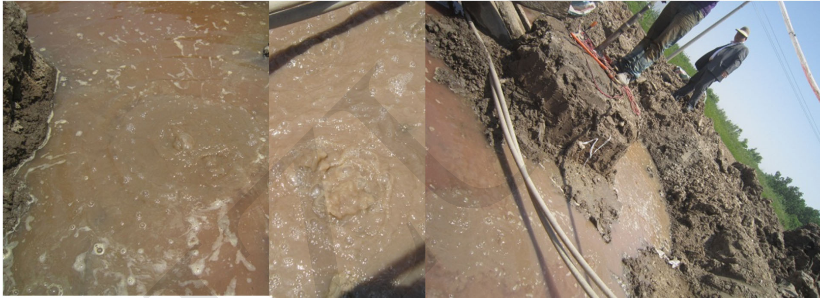
Fig. 4 Slurry breakout phenomenon of the in-situ slurry fracturing tests
