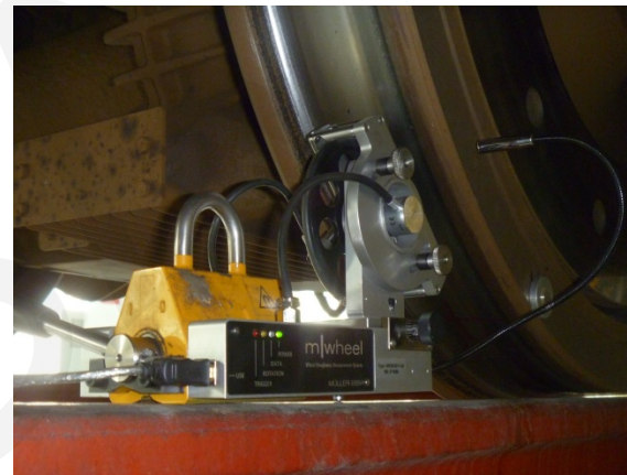
Fig. 2 Wheel roughness measurement
