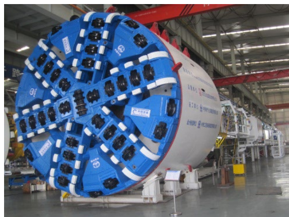
Fig. 1. Shield tunneling machine
