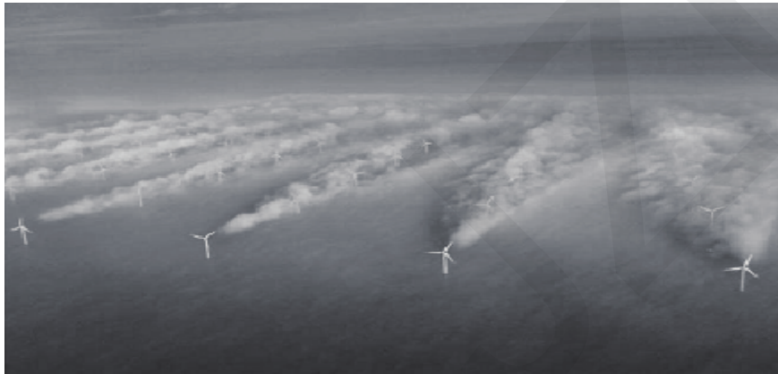
Fig.1 Wind turbine wakes in the wind farms [1]
