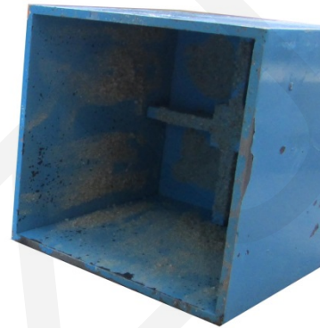
b) IBS footing with longer wall
