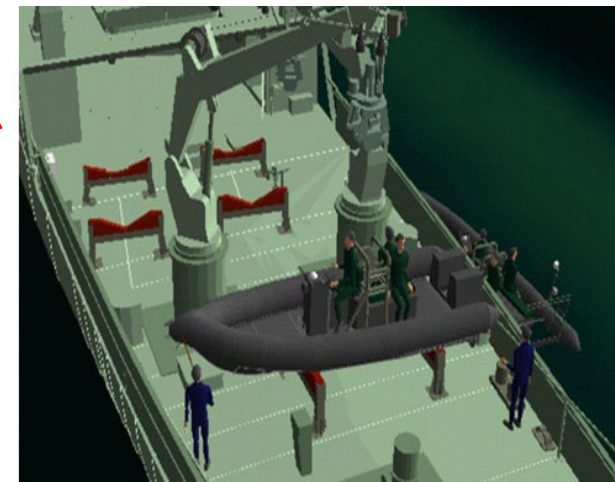
Fig.4 Launch and recovery of Rigid Hulled Inflatable Boats [1]
