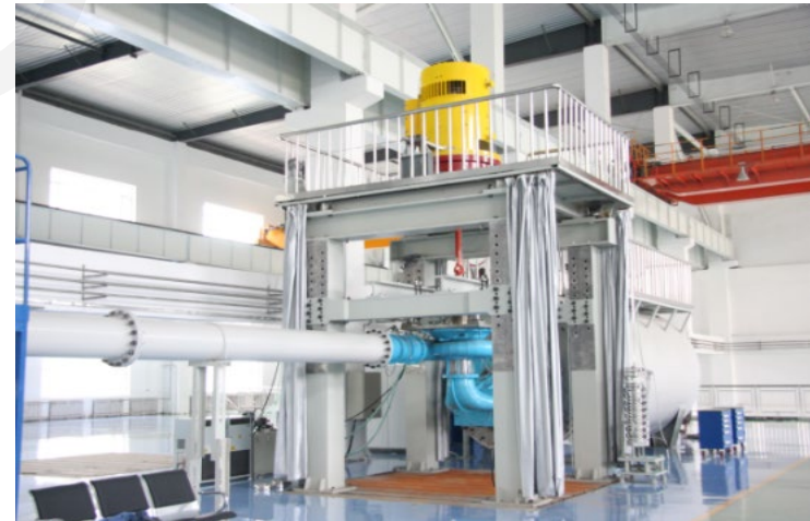
Fig.3 Test rig of a pump turbine model
