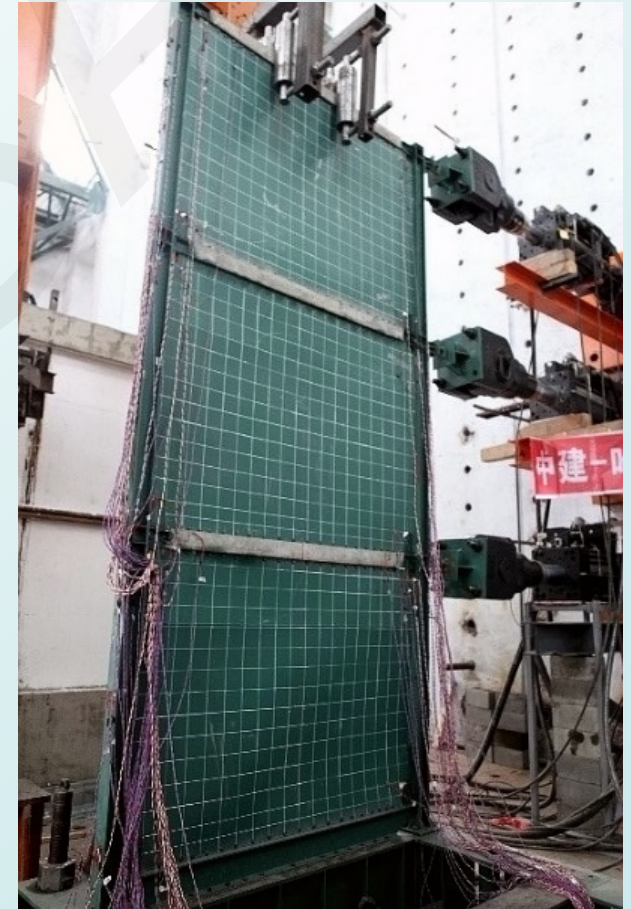
Fabricated composite frame with steel plate shear walls
