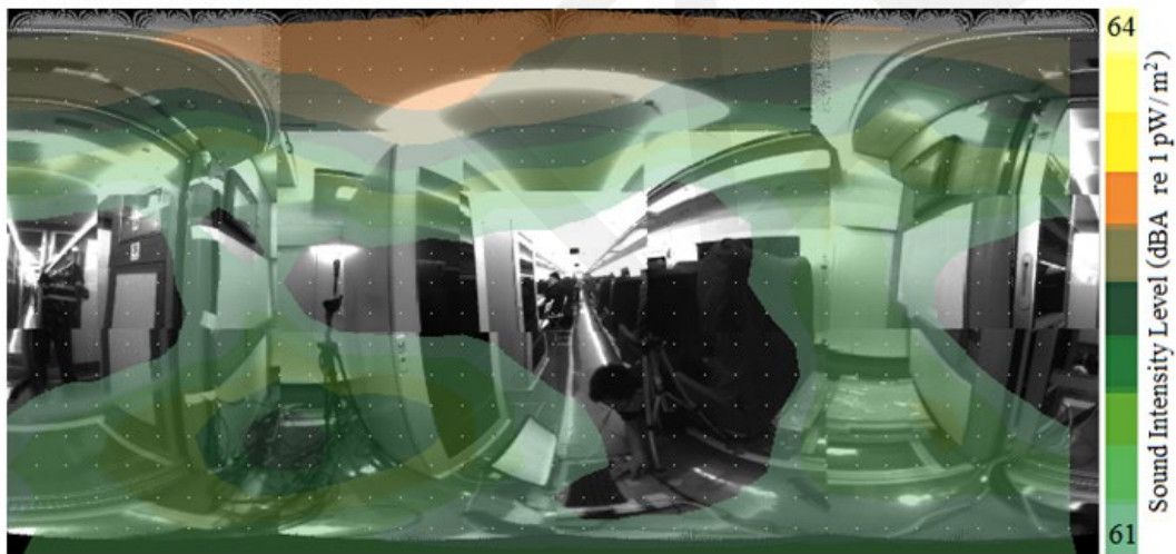
Fig. 15 Noise source identification result at the coach end of TP03 (50–5000 Hz)
