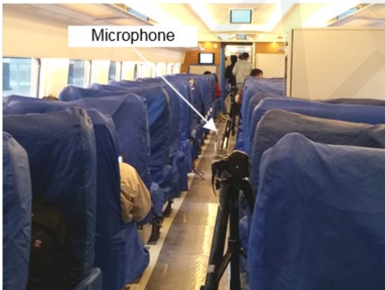
Fig. 1 Measuring points in the two coaches of a high-speed train (“•” refers to acoustic measurement points)
