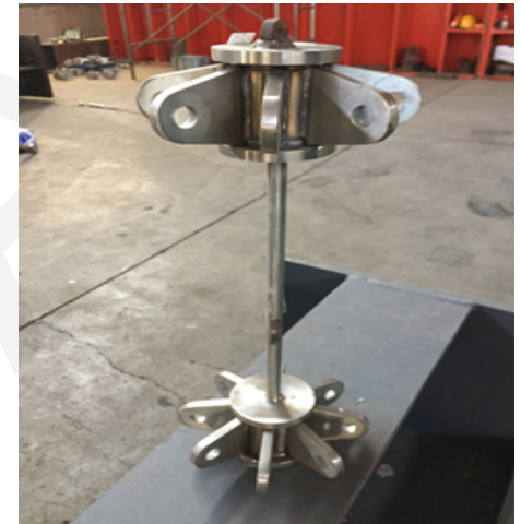
Lower joint of ST3
