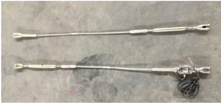
Cables with and without a tension sensor
