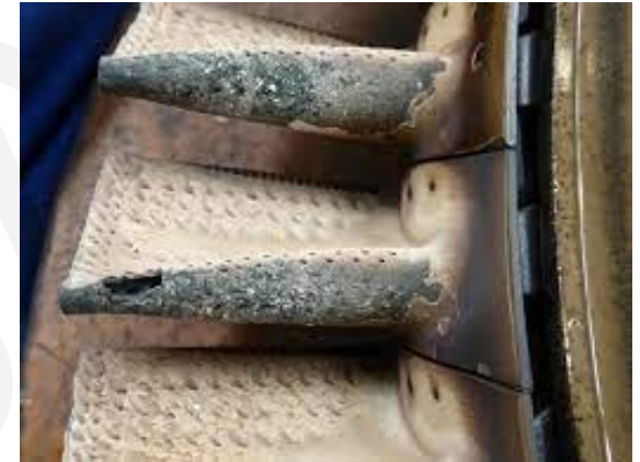
Damage in turbine blade
