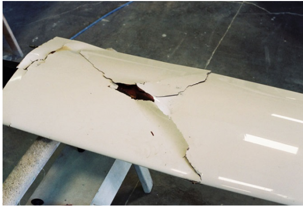
Damage in airplane wing
