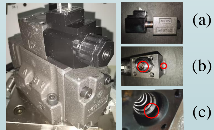
Fig. 3 Partial fault position of the directional valve; (a) electromagnetic fault location; (b) spring failure fault location; (c) valve body wear fault location
