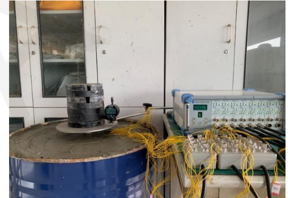
Fig. 6 Static load test equipment
