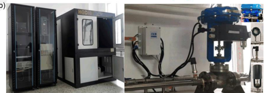
Figure (a) Mathematical model of pneumatic control valve; (b) The physical map of the test system: water hydraulic system, test control valve and sensors; (c) The control loop diagram of control valve
