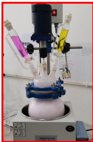
Preparation of \text{TiO}_2@\text{SiO}_2@\text{CeO}_2 with a reactor
