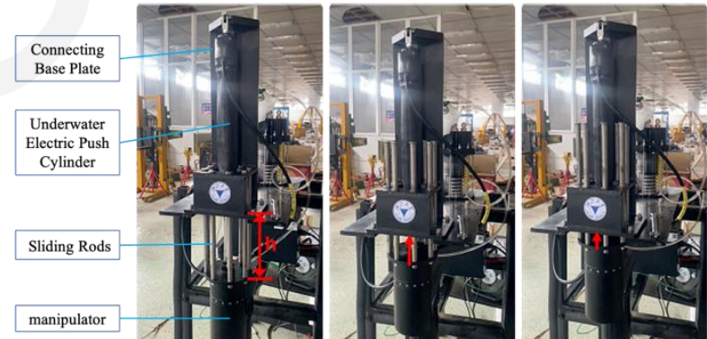
Display of the working process of the lifting mechanism
