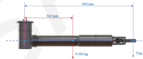
Upper Arm Joint Force Analysis Diagram
