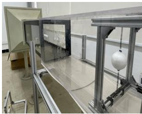
Experimental setup of the elastically-mounted sphere
