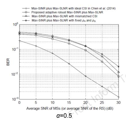
Curves of BER versus SNR of the proposed adaptive robust beamformer and existing non-adaptive ones ( $\Delta m f_d T_s = 0.01$ )
