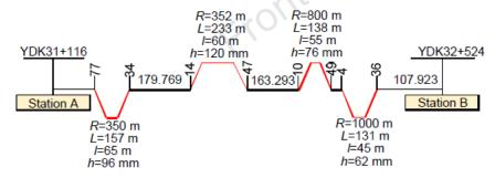
Fig. 14 Station A to station B: subway line curve information
