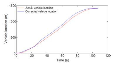
Fig. 17 Vehicle location after curve information correction
