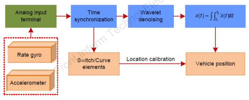
Fig. 5 Flowchart of vehicle location correction
