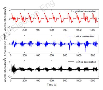
Fig. 10 Actual vibration accelerations of the vehicle body after coordinate alignment
