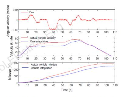
Fig. 16 Vehicle yaw angular velocity, speed, and location
